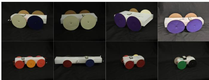
**Figure 2: The different fabricated 4-Wheeled and 6-Wheeled cars. Top Row: Designs evaluated in step pyramid environment. These had varying widths, with length, number of wheels and radius fixed; Bottom Row: Other Fabricated Designs, these had an assortment of different parameters.**
